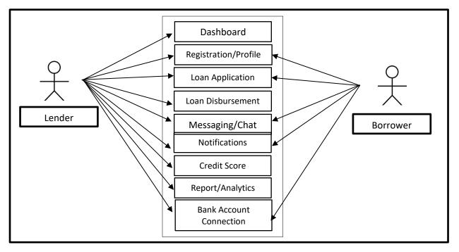
Shown above is the Online Lending System Use Case Diagram. The system has two user sides the Lender who will also act as Administrator and the Borrower of the system. The Lender can access the entire core modules of the system while the Borrower can access the Registration/Profile, Loan Application, Messaging/Chat, Notifications and Bank Account Connection modules of the system.
